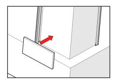
If utilizing Trim; connect the pieces around the Top and Bottom of the Post.
