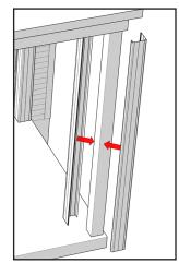
When snapping both pairs around the Post; ensure the Panels are square before finalizing the connection.
