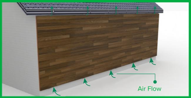
In order to allow air flow between the cladding and the wall, bottom and top ends should not be completely closed.
