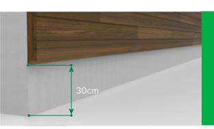
It is recommended to finish the cladding 30 cm (1 ft) above the ground. In this way, precautions will be taken against problems that may occur due to rainwater splashes or snow level height.
